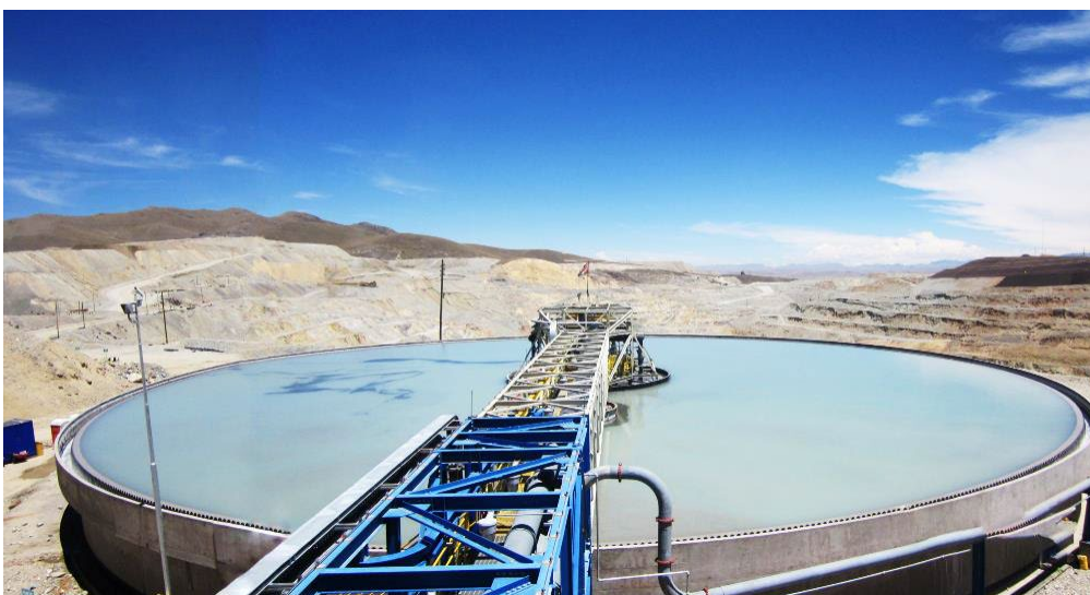
A DELKOR High-Density Thickener installed in Peru with a 60 m diameter, similar to the equipment being supplied for Talabre.
