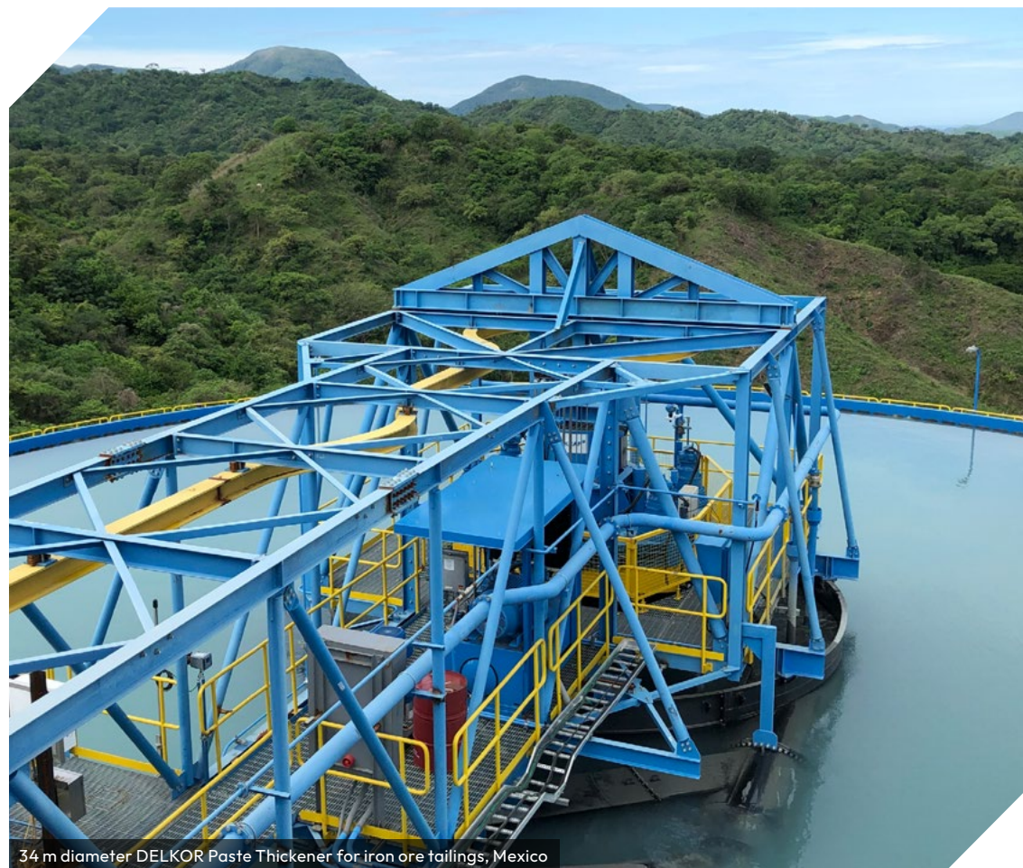
34 m diameter DELKOR Paste Thickener for iron ore tailings, Mexico
