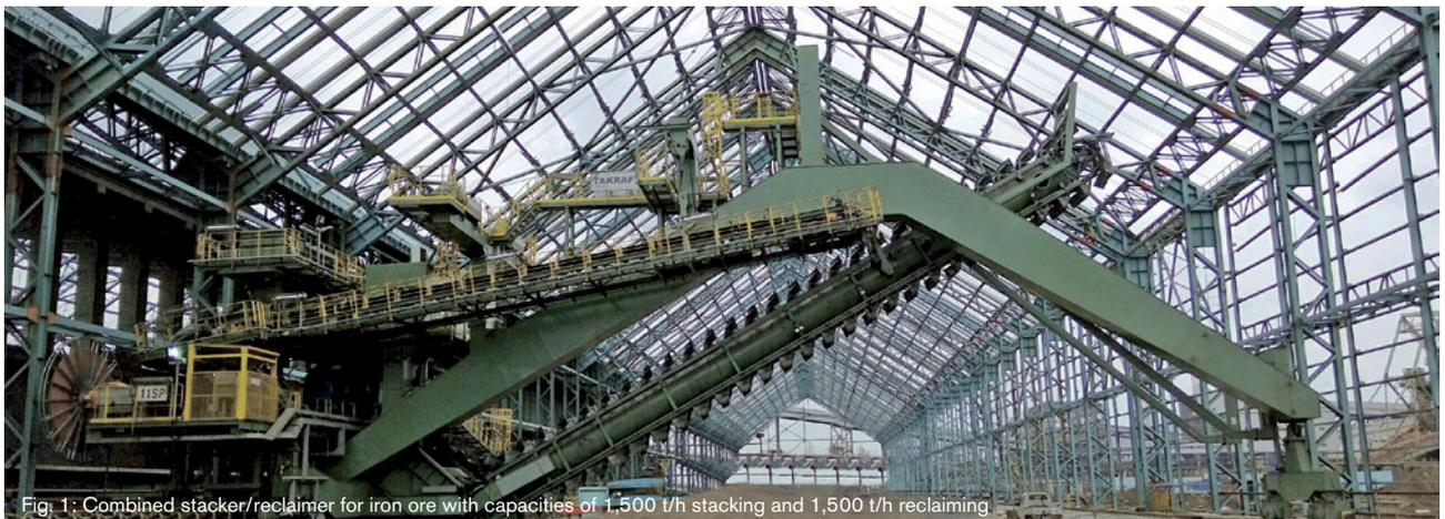
Fig. 1: Combined stacker/reclaimer for iron ore with capacities of 1,500 t/h stacking and 1,500 t/h reclaiming
