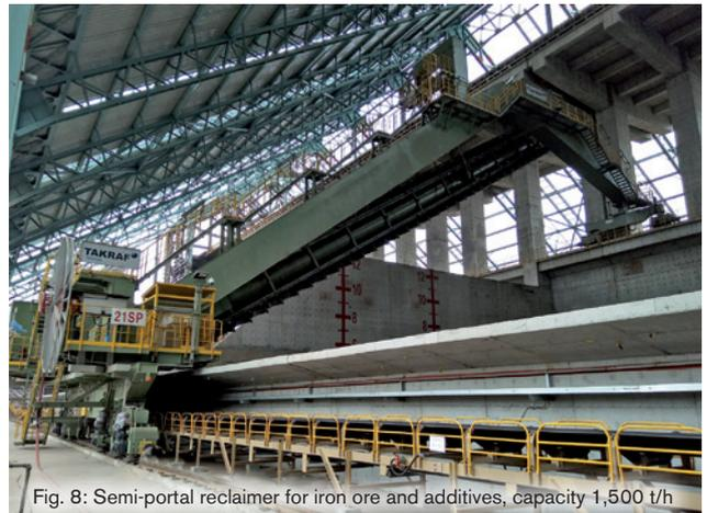
Fig. 8: Semi-portal reclaimer for iron ore and additives, capacity 1,500 t/h
