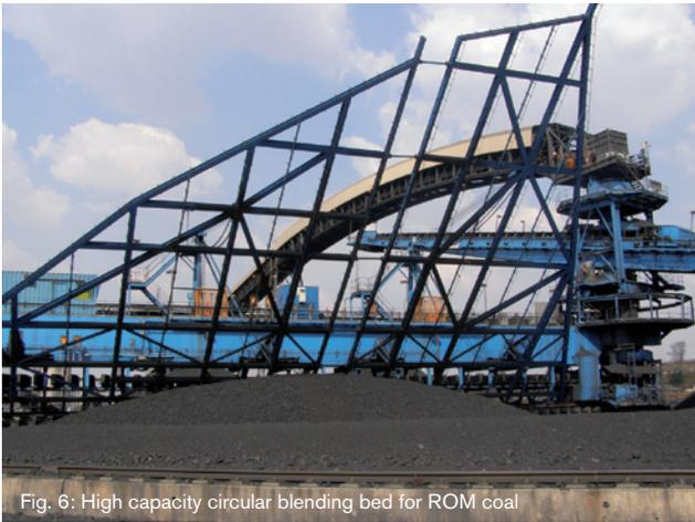
Fig. 6: High capacity circular blending bed for ROM coal
