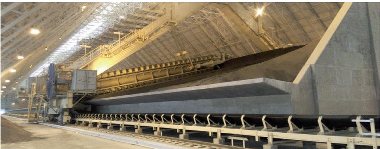
Photo above: Portal reclaimer in a phosphate product storage facility boasting a 51.7 m rail span and a 2,000 t/h capacity
