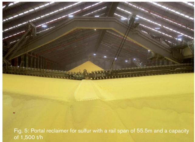
Fig. 5: Portal reclaimer for sulfur with a rail span of 55.5m and a capacity of 1,500 t/h
