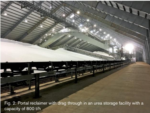
Fig. 2: Portal reclaimer with drag through in an urea storage facility with a capacity of 800 t/h
