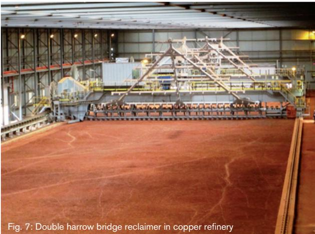
Fig. 7: Double harrow bridge reclaimer in copper refinery
