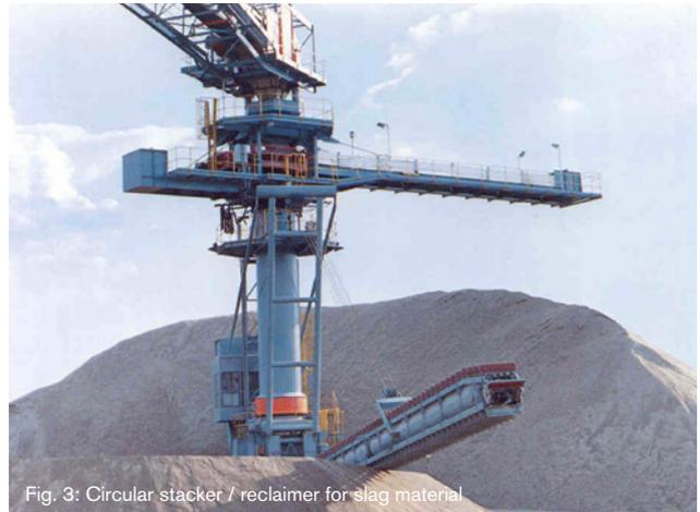
Fig. 3: Circular stacker / reclaimer for slag material
