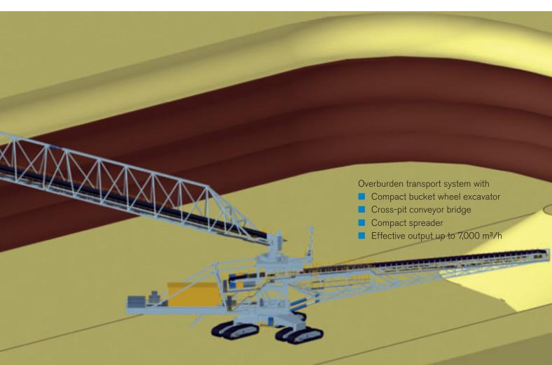
Up to 240,000 bank  $\rm m^3$  of overburden per day can be shifted in cross-pit operation using various combinations of our machines.
