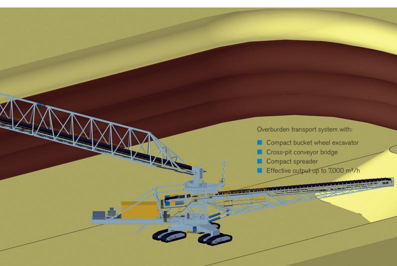
Up to 240,000 bank m<sup>3</sup> of overburden per day can be shifted in cross-pit operation using various combinations of our machines.
