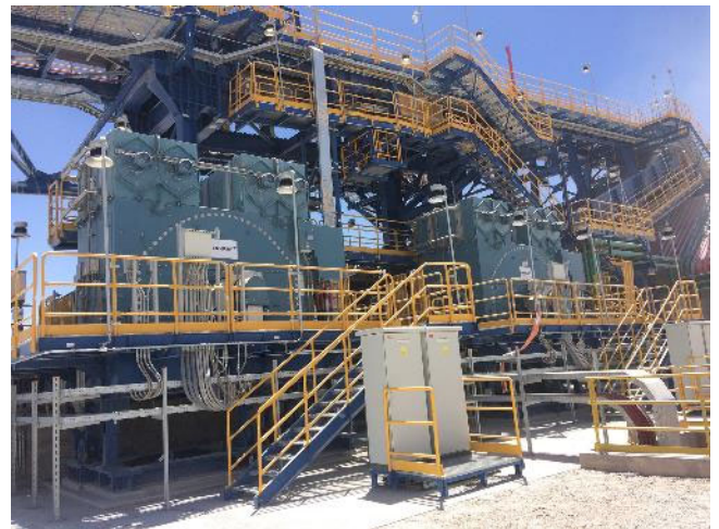
Caption: Advanced gearless drive technology was applied in the design of the world's most powerful conveyor system at Chuquicamata in Chile.
