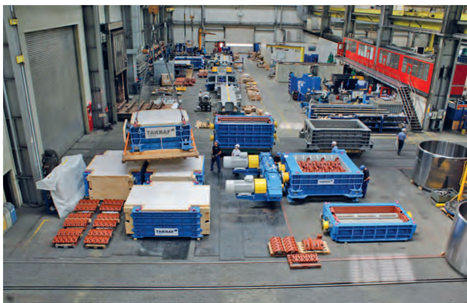
TAKRAF sizer pre-assembly at the factory
